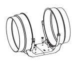
3. Secure the mount with screws in your desired location.
